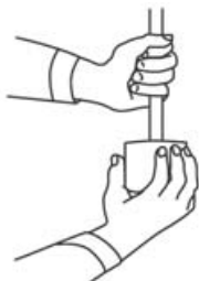
Fig. 15 Cleaning off burrs (reaming)
